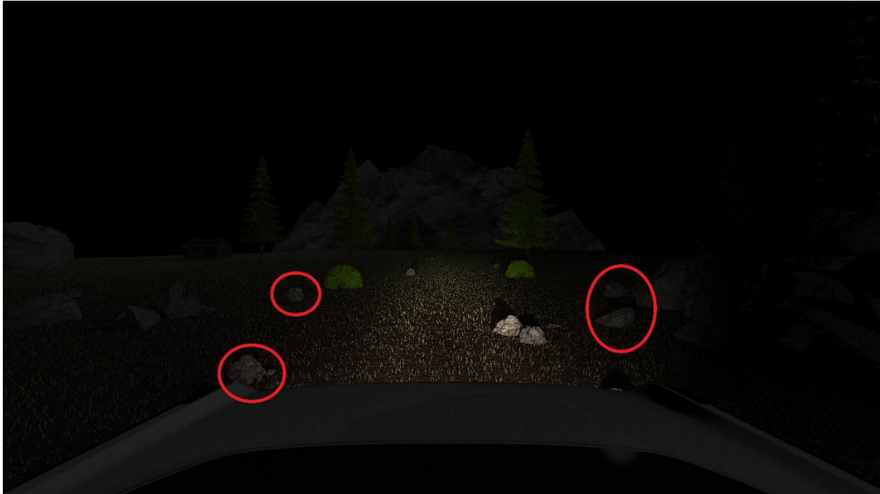
Picture 8: Rendering of a pair of Baja Designs S1 Spot lights (Zone 4, Blend Angle 72°, Blendability 6.1) created from .IES test measurement files. Notice the illuminated objects in the transitional light outside of the bright center beam (circled in red) then refer to Picture 9 showing pair of Diode Dynamics SS1 Pro Spot lights in the same environment.
